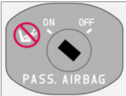
Switch for SRS in ON position.
